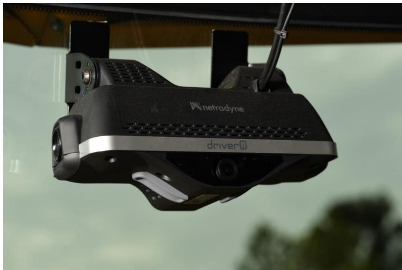
Netradyne uses artificial intelligence (AI) vision-based dashcam devices to monitor safety performance of fleet vehicles. Netradyne's system may also crowdsource road and driving behavior metadata.
